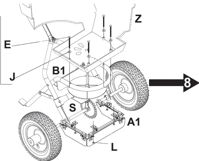
**Important:** Adjust bracket on the gear(S) and ensure that the deflector (A1) flaps are pulled down before installation.
