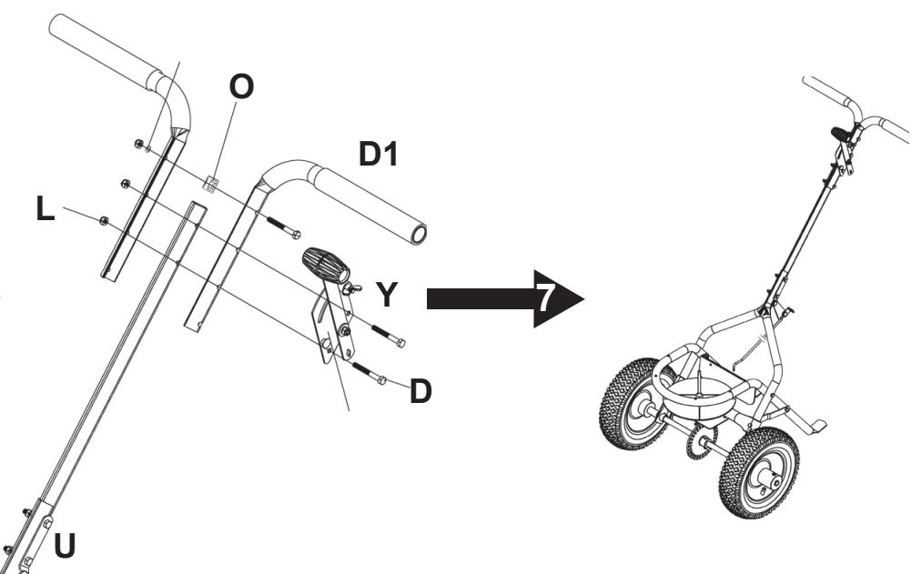
Insert spacer (O) onto the upper hole of the handle rod (U). Attach the bolt (D) onto handle (D1), secure with nut (L). Now tighten the other bolts to secure the handle.
