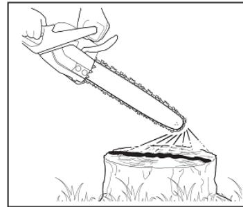
**⚠ Always check that the machine is filled with chain oil before starting. Operation without chain oil can cause damage to the saw.**
