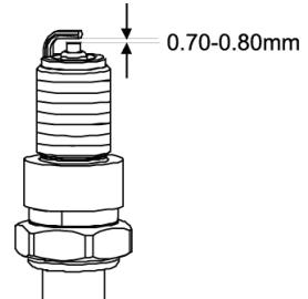
**Note:** The engine must be cold
